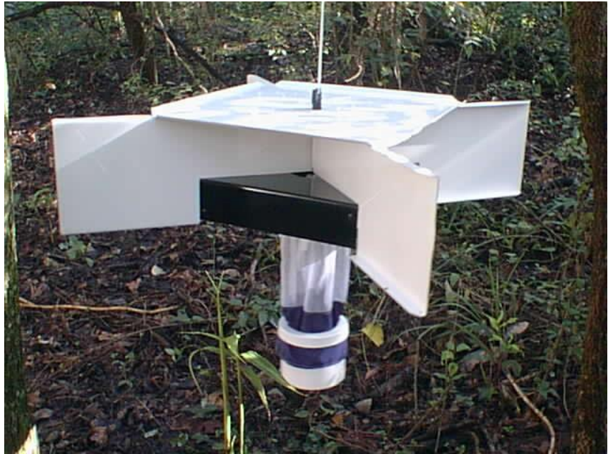
Figure 1. Omni-directional Fay Prince trap with collection cup.
