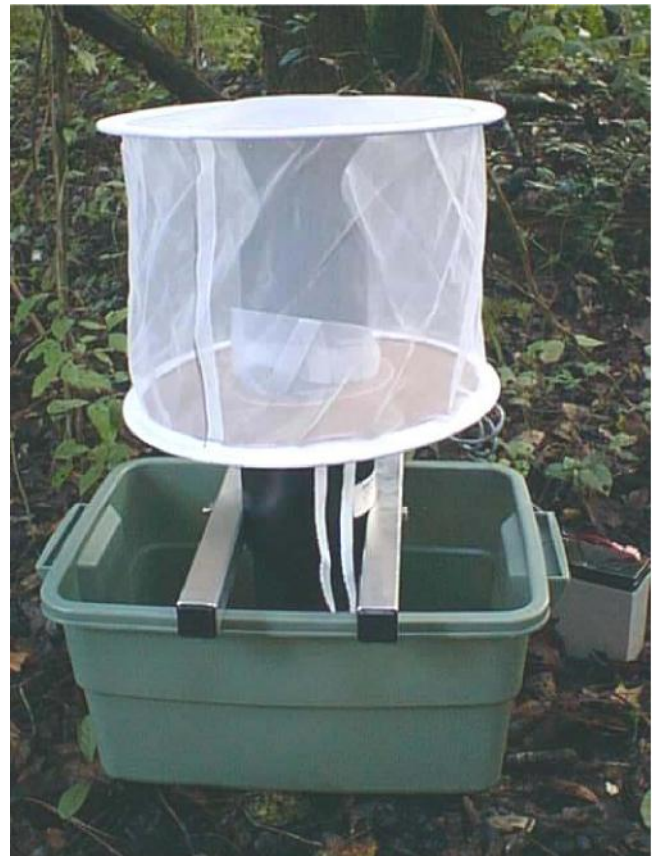
Figure 1. The CDC Gravid Trap with a 6 Volt, 10 AmpHr battery.
