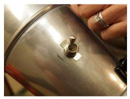
The final switch (3) is the operational switch used to permit or to stop the motor from running. It is conveniently located on the stainless steel collection bell which holds the collection bag (image on left). It is labeled ON and OFF.
