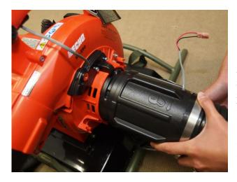
Align the intake tube with the locked and unlocked icons on the black tube to the right and left of the black index boss on the intake housing, as shown on left. Next press the intake tube into the motor housing and turn the tube to the right (clockwise) until it will turn no further. If the tube should come out during operation, there is a switch within the motor housing at this location that will shut off the ignition and the motor will stop.
