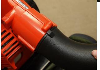
The image to the left shows the exhaust tube correctly inserted into the orange exhaust housing of the motor.
