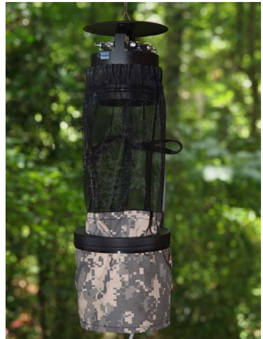
Figure 1. The new Stealth Trap, Model 2014. Included items are the trap, collection cup and sock, and the battery connector and adapter for all types of batteries.
