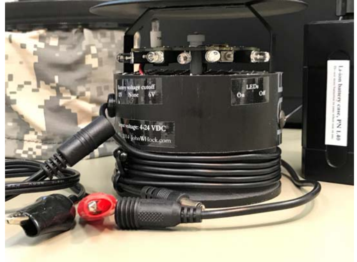
Figure 2. The Stealth Trap Model 2014 showing battery voltage cutoff switch and LED on/off switch. On the opposite side from the LED switch is the incandescent light off/on switch. Also shown is the trap's battery connection (5.5 x 2 mm barrel connector for the Li-ion battery box); also shown is the adapter cable that allows attachment of the trap to virtually another type of battery. To the right of the trap is the Li-ion battery box (PN 1.40).
