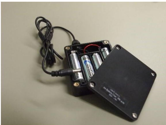
Figure 2. Waterproof battery box and connecting power cord.
