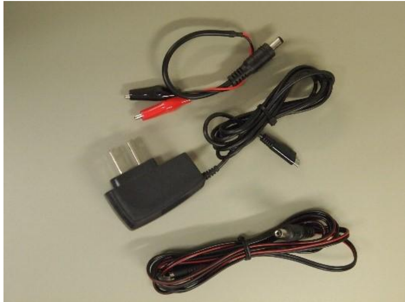
Figure 3. The items are from top to bottom: a. insulated alligator clips to permit the use of any six-volt battery, b. 100-240 AVC/ 50-60 Hz adapter, and c. an extension cord that can be used to extend the distance between battery and/or adapter and the aspirator. All connections are barrel connectors, 5.1 by 2.1mm.
